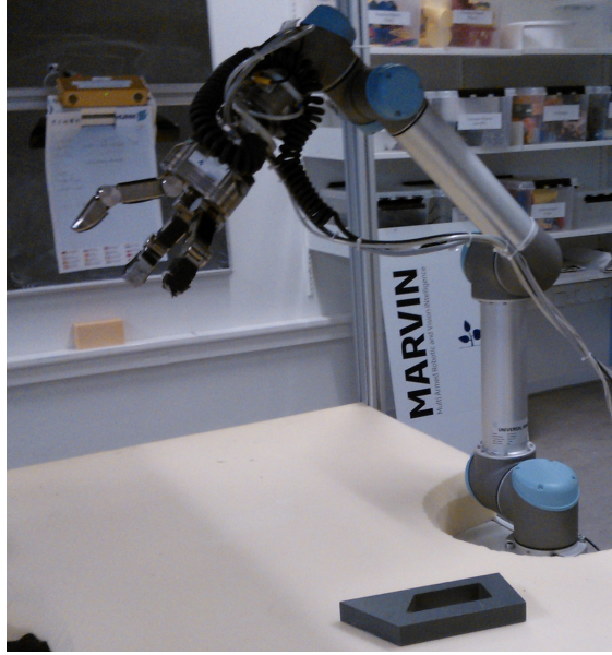
Figure 10: The UR-6-85-5-A robot arm mounted with a Schunk Dexterous Hand (SDH). The object in the lower right corner is the Rump object.
