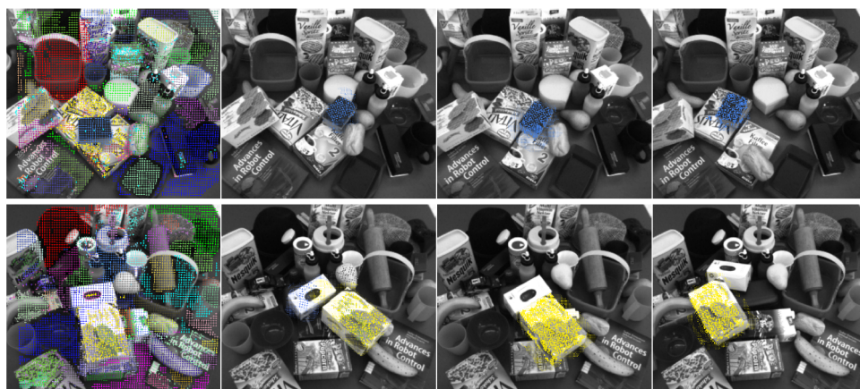
Figure 3.2: Interactive segmentation of unknown objects in clutter: The left image in each row shows the initial object hypotheses, the following images show the segmentation results after one, two and three pushes respectively.
