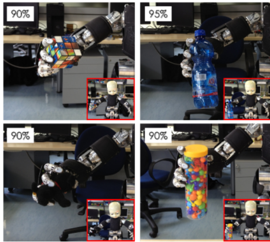
Fig. 6. Objects used to test our method with their respective success rates over 20 trials.
