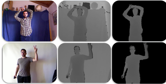
Figure 2: Region of Interest detection. Left: RGB video frames. Center: depth frames. Right: the detected ROI.
