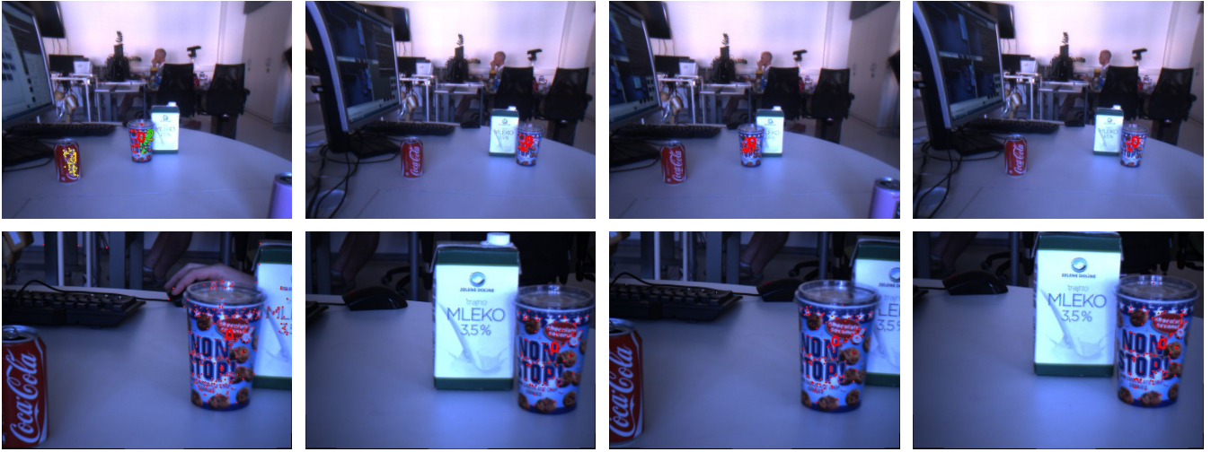
Fig. 3. A typical object learning / recognition procedure. The upper row respectively shows the peripheral and the bottom row the foveal view. The images in the first column contain the initial object hypotheses as the head is turned towards hypothesis "0". Each of the following columns shows the scene after moving the object, validating the initial hypothesis and accumulating the verified feature points for learning or recognition.
