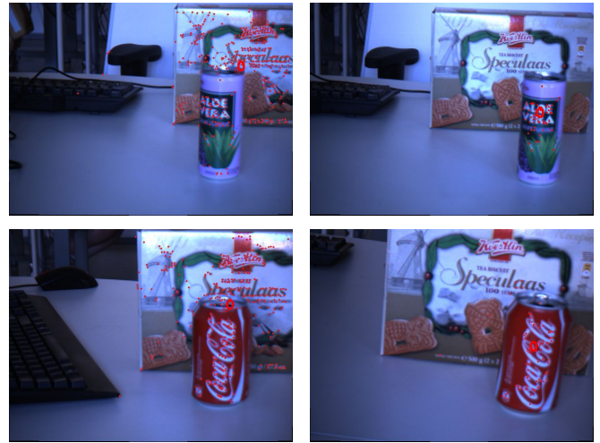
Fig. 4. In the first row, the initial hypothesis in the foveal view is validated with the rigid body motion filter and in the second row with the static feature filter. The rigid body motion filter discards all the background features and all false matches. The static feature filter requires a static background and cannot filter false SIFT matches.
