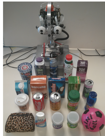
Fig. 1. Karlsruhe Humanoid Head [13] and the object test set used in the experiments. The head is equipped with two cameras in each eye. One pair of cameras models human peripheral vision, the other pair foveal vision.
