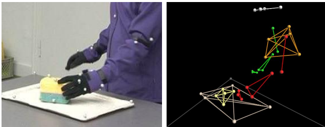
Fig. 2. Left: Human demonstrator with markers attached to him and all objects while wiping a tray. Right: The same frame of the demonstration as the 3D view of the reconstructed marker groups (different colors).
