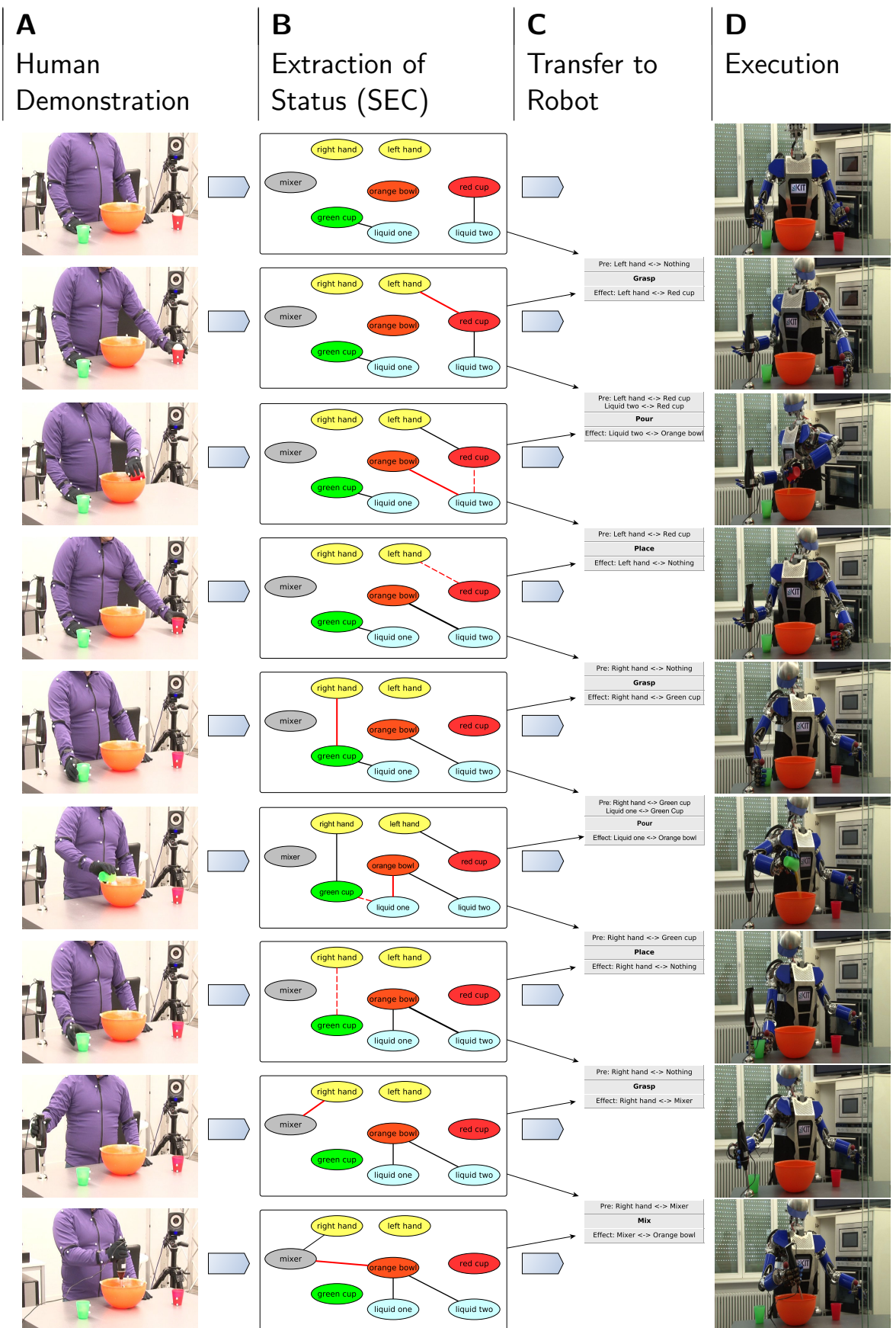
Figure 2.7: Transfer of action knowledge from human to robot. A) Human demonstration, B) SEC depicted by ways of its key frame graphs, which show which objects touch which other objects (edges) during human execution. C) Abbreviated Executables D) Robot execution.
