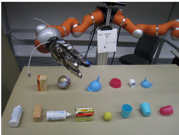
Fig. 4. The experiment setup. Kuka LWR robot arm and Schunk gripper are used for manipulation and Kinect is used to extract object features including object's position. The environment includes one and two objects during single-object and multi-object affordance learning experiments, respectively.
