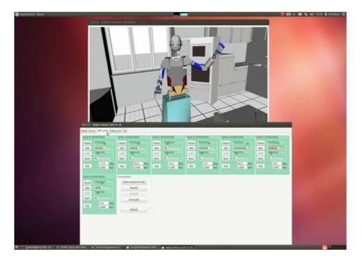
Figure 1.4: Controlling the ARMAR-III robot (simulator) using the YarpMotorGui.
