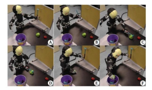
Figure 3.4: The iCub performing table-cleaning using a tool (rake). The robot take the tool (A), reaches for the object (B,C), pulls the object (D), grasps the object (E) and finally places it into the bucket (F).
