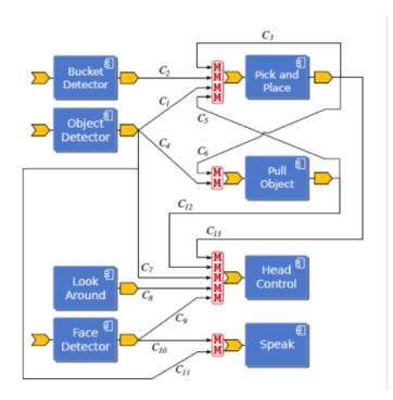
Figure 3.3: Configuration of the modules for table-cleaning application.
