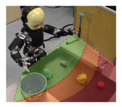
Figure 3.2: The experimental setup of table-cleaning application. The reachable zone is depicted in green, the orange zone represents the zone reachable with the tool and finally the red zone indicates the unreachable space, for which the robot needs human intervention.
