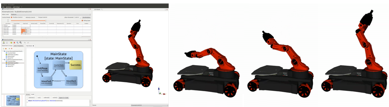
Figure 12. The waving statechart executed on YouBot, while running a kinematic simulation.
