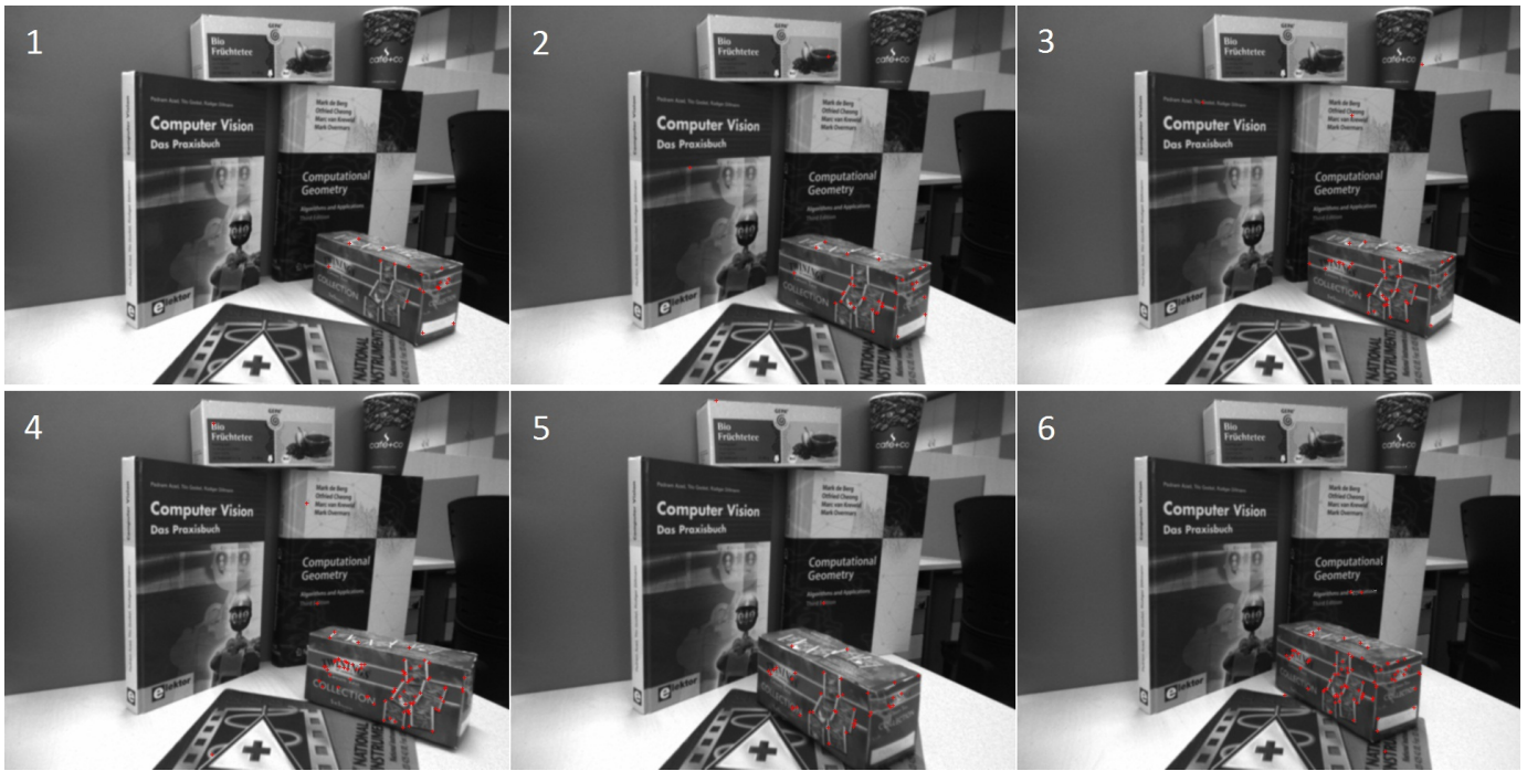
Fig. 4. An object is learned by accumulating verified feature points on its surface during repeated pushing. At each step, new candidate points are added to the object hypothesis and verified after the next push.
