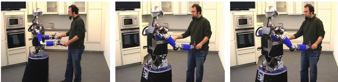
Figure 2.2: Coaching of the humanoid robot ARMAR-III via kinesthetic guiding
