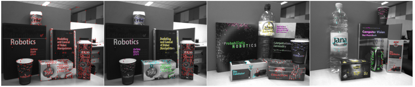
Fig. 2. Hypotheses generation: The left image shows all detected Harris interest points, the other images display the generated hypotheses for each scene. Usually, the hypotheses correspond to a textured region on an object's surface. When objects are close to each other and points on their surfaces lie on a common plane or cylinder, it may happen that these points are subsumed in one hypothesis.
