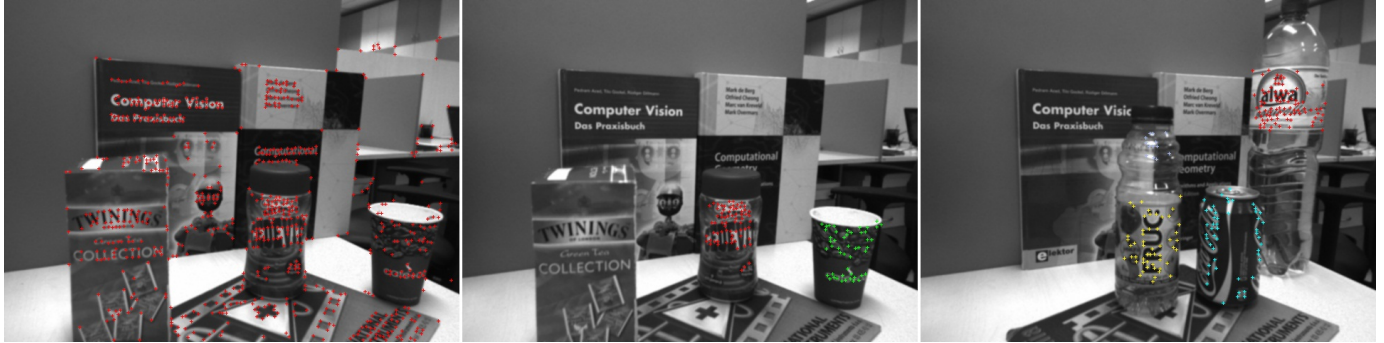
Fig. 3. Hypotheses generation for cylindrical surfaces. The left image shows all Harris interest points, the central and right images show the generated cylindrical hypotheses. Although the two objects in the central image do not have an exactly cylindrical shape, a large part of their surfaces can be captured by the cylinder hypotheses.
