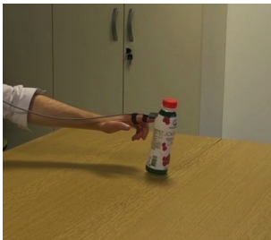
Figure 2.1: Data acquisition for the extraction of push affordances. A magnetic tracker is attached to the finger.
